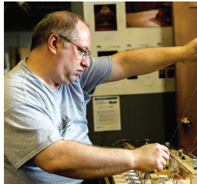
Wiring the valve-opening mechanism. Beneath each pipe in the windchest is a solenoid, which, when energized, opens the valve to allow wind to flow into the pipe. (Peragallo)
