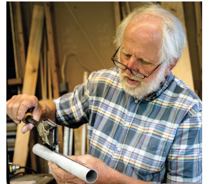
Soldering the seam on a metal pipe. With the exception of the seam area, the pipe is coated with “size”—a mixture of ground calcium carbonate and gum arabic. The solder does not adhere where the pipe is coated with size. (Moore)
