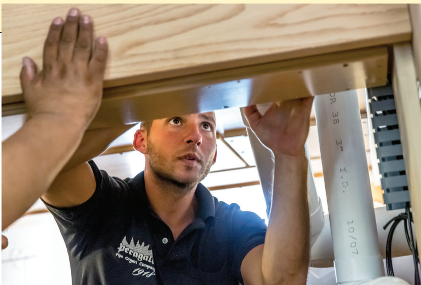
Lining up the wind line for a façade chest (Peragallo)
