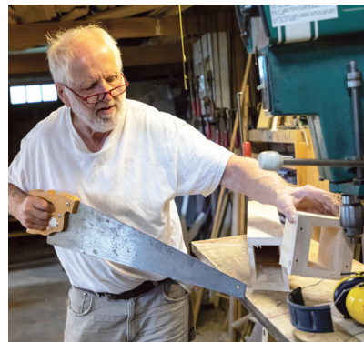
Cutting an air trunk. The chop saw was able to get through about 90% of the windtrunk. The job is finished with a handsaw. (Moore)
