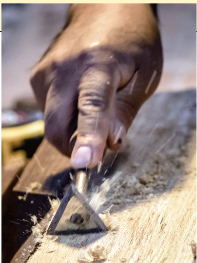
Preparing wood surface with a scraping tool (Peragallo)
