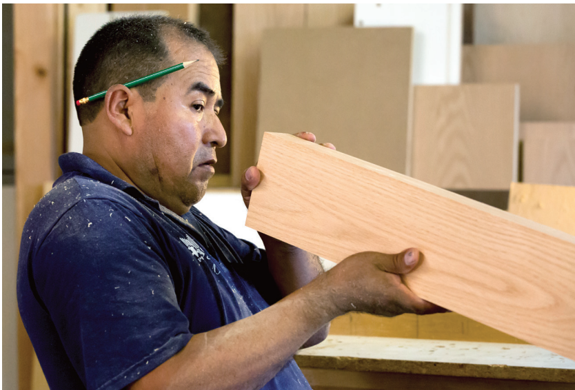
Checking a piece of lumber for straightness (Peragallo)
