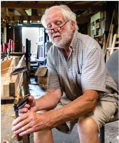
David Moore clamping up a 16' Trombone, a wood reed stop. This is a replica of a stop in an E. & G. G. Hook organ.
