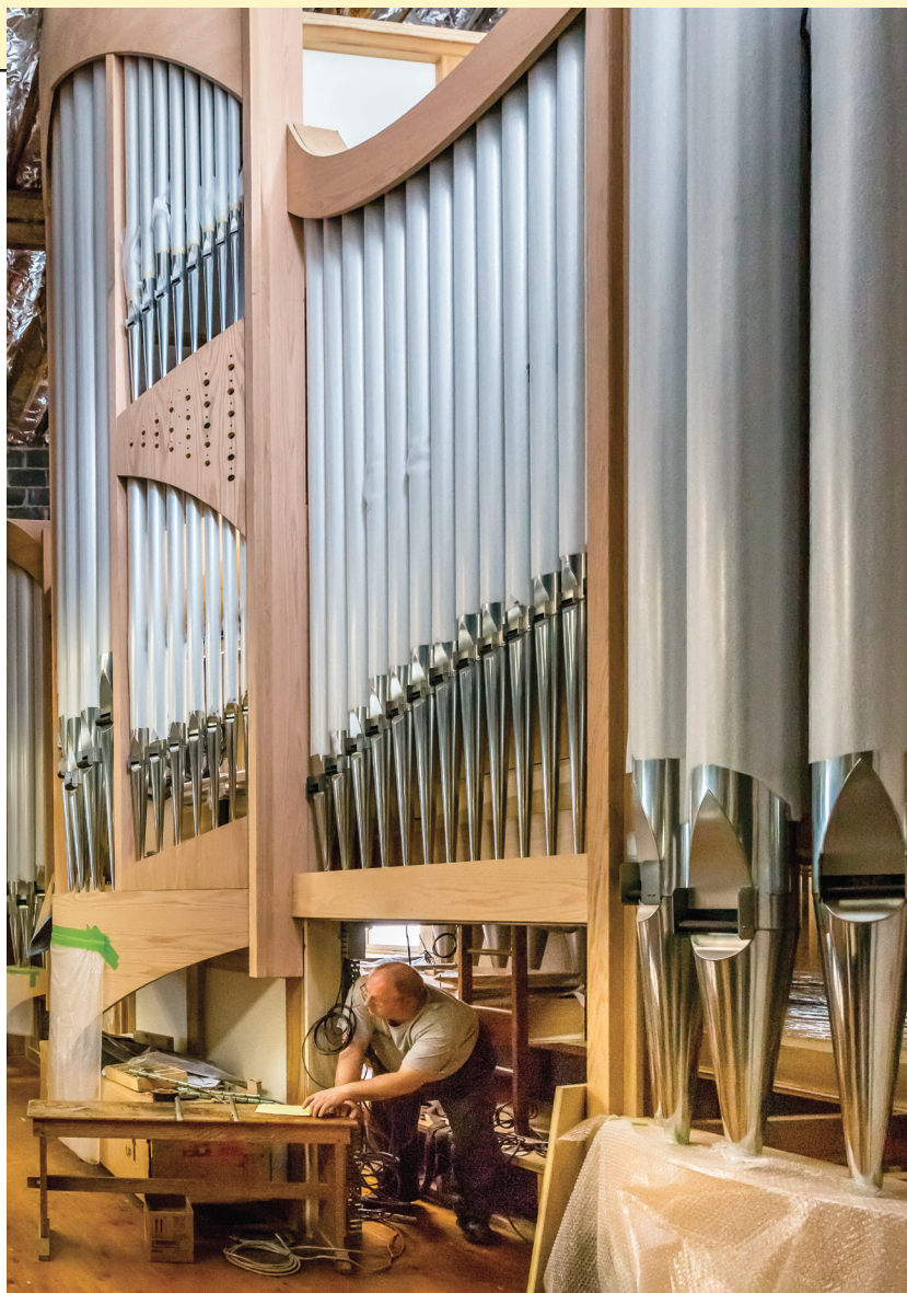
Emerging from the case of the Cathedral of Saints Simon and Jude instrument after a session of switching circuit wiring (Peragallo)
