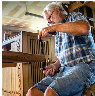
Rounding the end of a wooden reed pipe using a draw shave (Moore)
