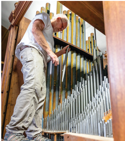
Tuning the Hook & Hastings in the erecting room. This is a stock model two-manual instrument dating from around 1910. (Moore)
