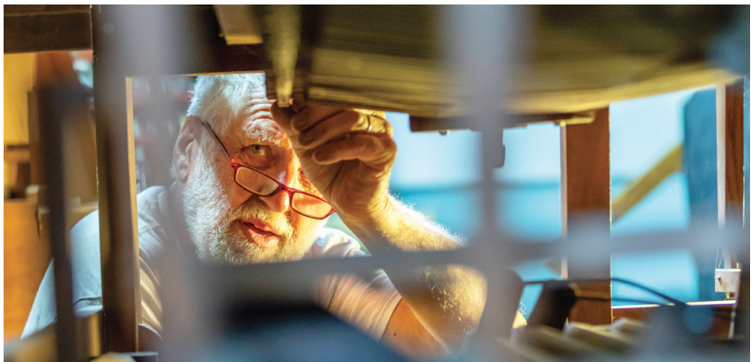
Adjusting the key action on the Hook & Hastings organ (Moore)
